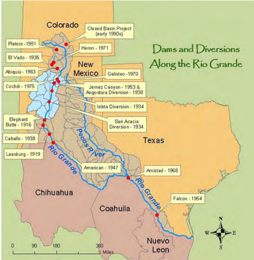
Figure A4.4. Dams and diversions along the Rio Grande. 27
